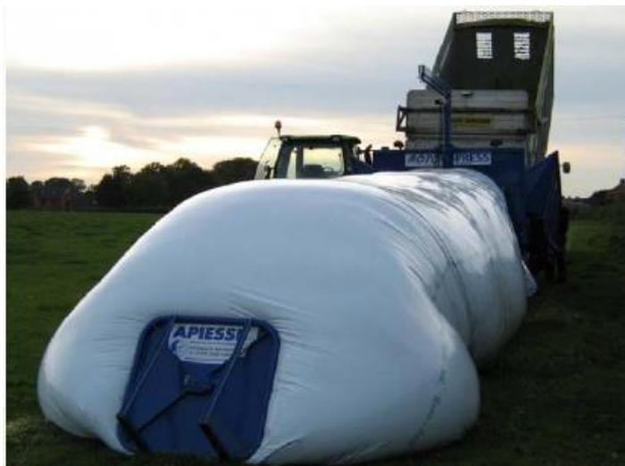
**Figure 21** Plastics silage bags made by Roto-Press [307].
