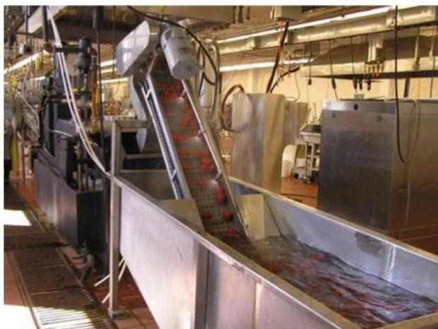
**Figure 6** Tomato washing in a tank before transporting to the lye peeler.
